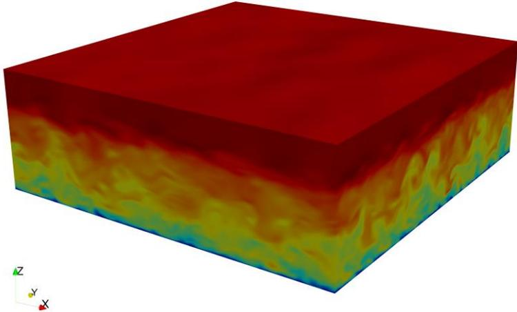
Velocity field in a representative AMR-Wind large-eddy simulation of a  $3 \times 3 \times 1 \text{ km}^3$  domain for a neutrally stable ABL
