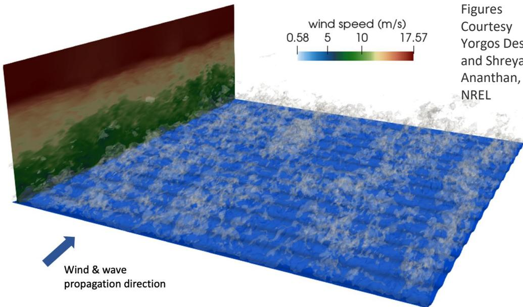
LES of a marine atmospheric boundary layer over idealized, wind following and fast-propagating long waves (swell)
