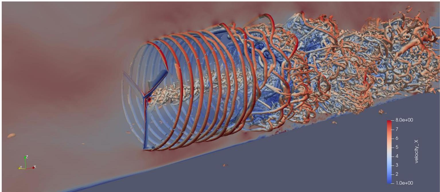
Visualization of the flow field around the 2-MW NM80 wind turbine under turbulent inflow. The isosurfaces highlight vortical structures and the colors indicate streamwise velocity.
