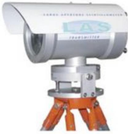
Large Aperture Scintillometer (LAS): several km, visible / IR
